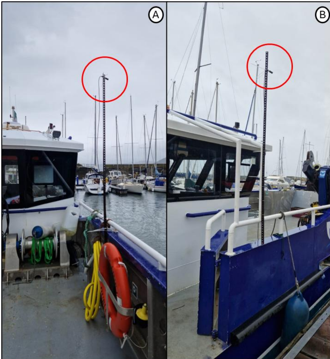
Figure 2-4: Placement of the microphones on the starboard side (A) and the port side (B) of the vessel
